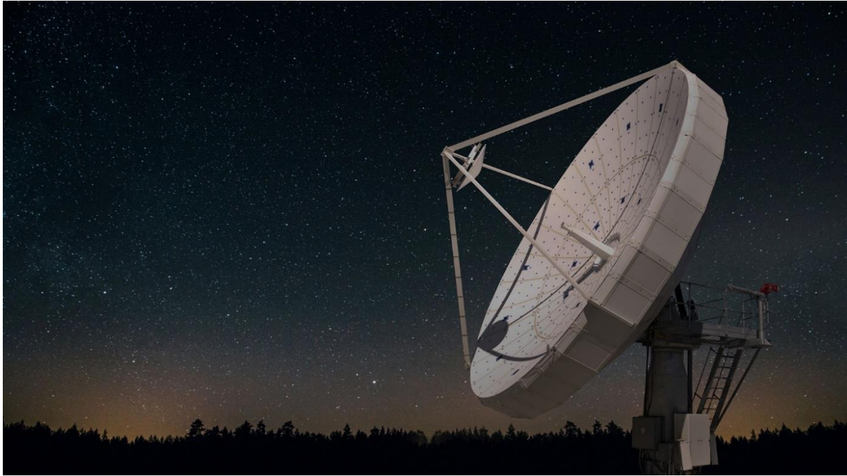
Figure 2. A Ka-band satellite gateway antenna used in Viasat's government/military SATCOM systems. Source: Viasat. 16
